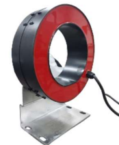
TRANSFORMADOR TOROIDAL 50-100/1A, 1VA, 5P20
